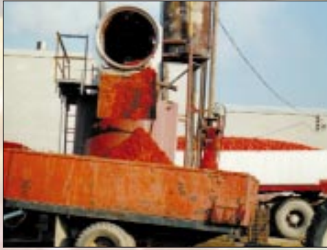
Produce operation doing tomatoes, potatoes, mushrooms, etc. Lye peeled tomato operation shown. Operation is accomplished without backwash. There is very little free water with the solids — note the peak of the solids.
