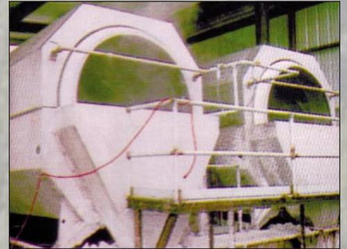
Two MDS units installed to wash and thicken the fibre from 1.5 to 3%, 12 to 16% out.
