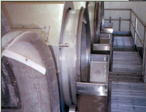
Secondary (WAS) sludge thickening system increasing solids from <1% to 8%+ prior to hauling for disposal. Polymer consumption for this type of application is typically 4 to 9 lbs/ton of dry solids as a function of the sludge.
