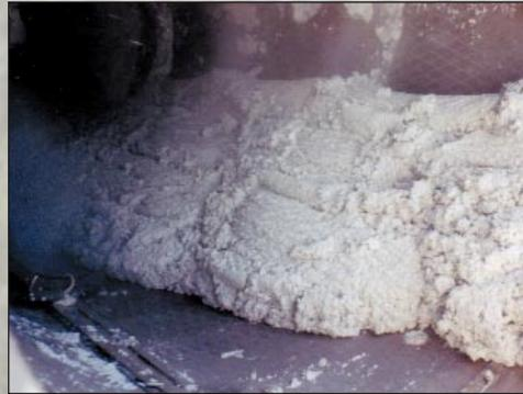
The de-inking sludge comes off of flotation clarifiers at 2–3%, with as much as 40% clay or ash. The solids come off our MDS at 12 to 15 to 18% allowing the press to meet its goal.
